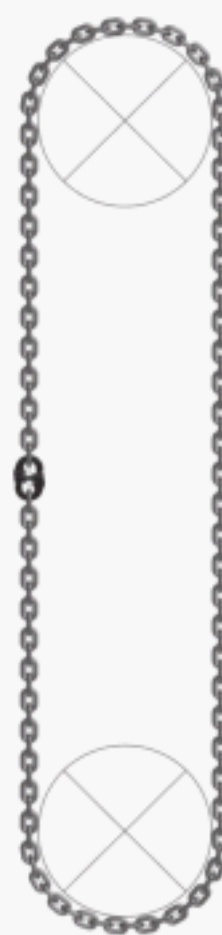
(f) Endless Sling, Straight-Line Hitch
