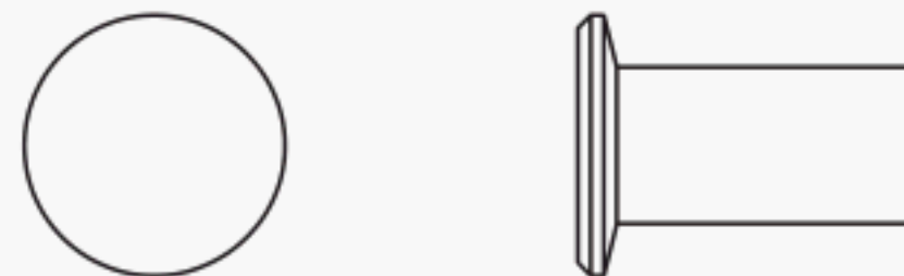
Flat Top Countersunk Head (With Chamfered Top)
