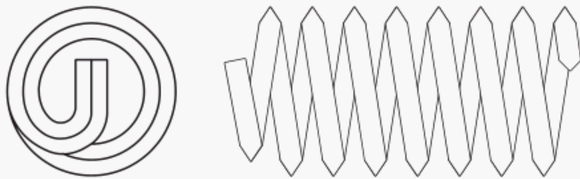
Helical Thread Insert
