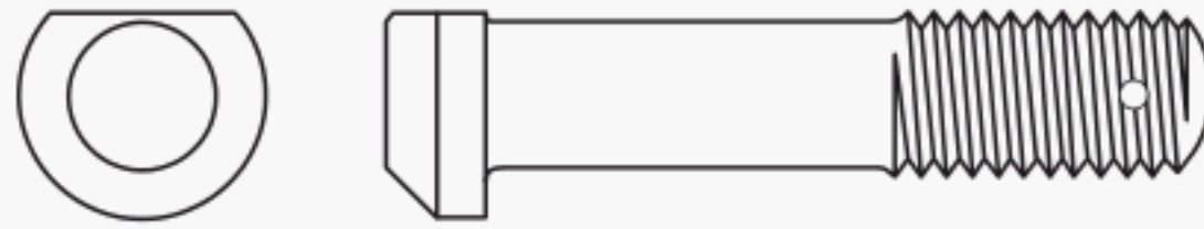
Connecting Rod Bolt
