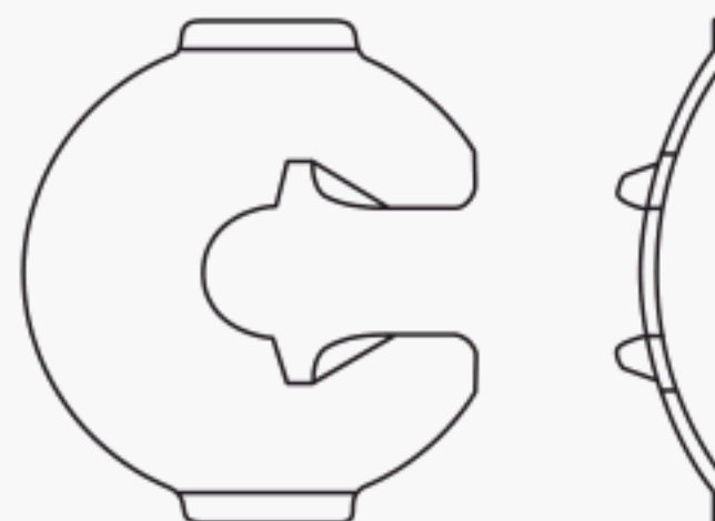
External Bowed Locking Prong Ring (Type NA16)
