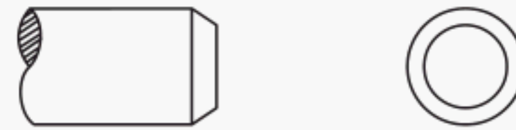
Chamfer Point
