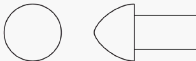
High Button Head Large Rivet
