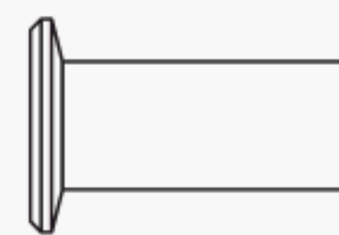
Flat Top Countersunk Head Tubular Rivet (With Chamfered Top)
