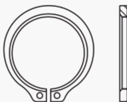
Beveled External Ring (Type NA12)
