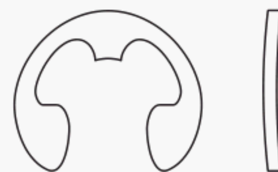
Bowed E-Ring External (Type NA9)
