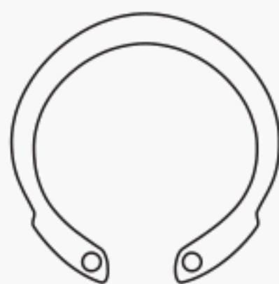
Inverted Internal Retaining Ring (Type NA11)
