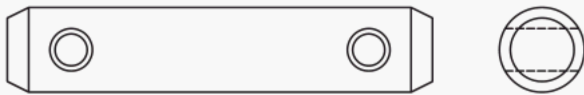
Headless Clevis Pin
