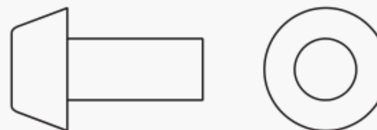
Boiler Rivet
