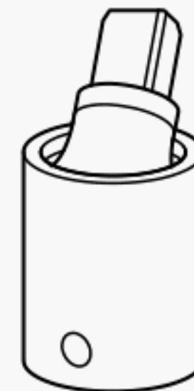
FIG. 5 TYPE VI, UNIVERSAL JOINT
