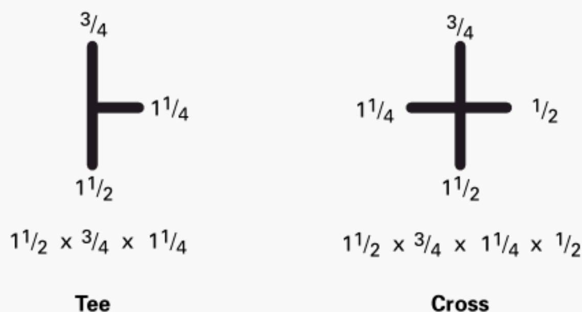
Fig. 1 Method of Designating Outlets of Reducing Tees and Crosses
